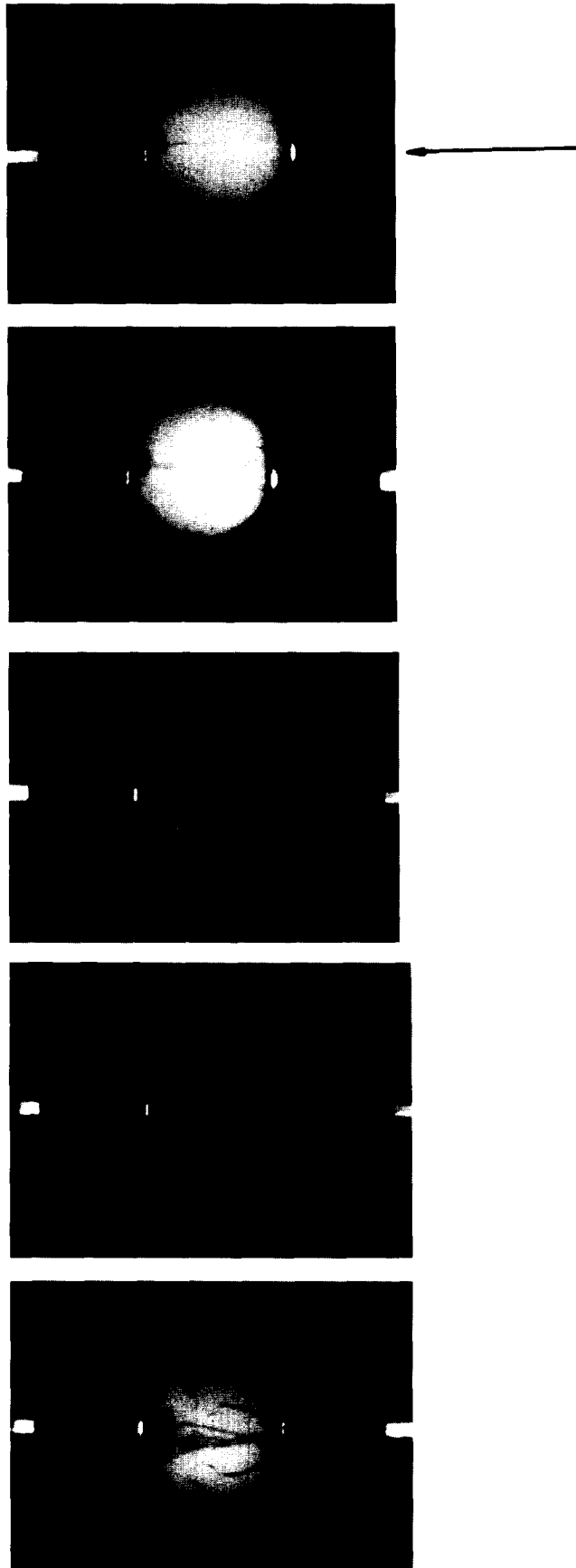
Fig. 3. Glass-ceramic disc under dynamic diametral loading. Framing interval, 0.01 ms.
